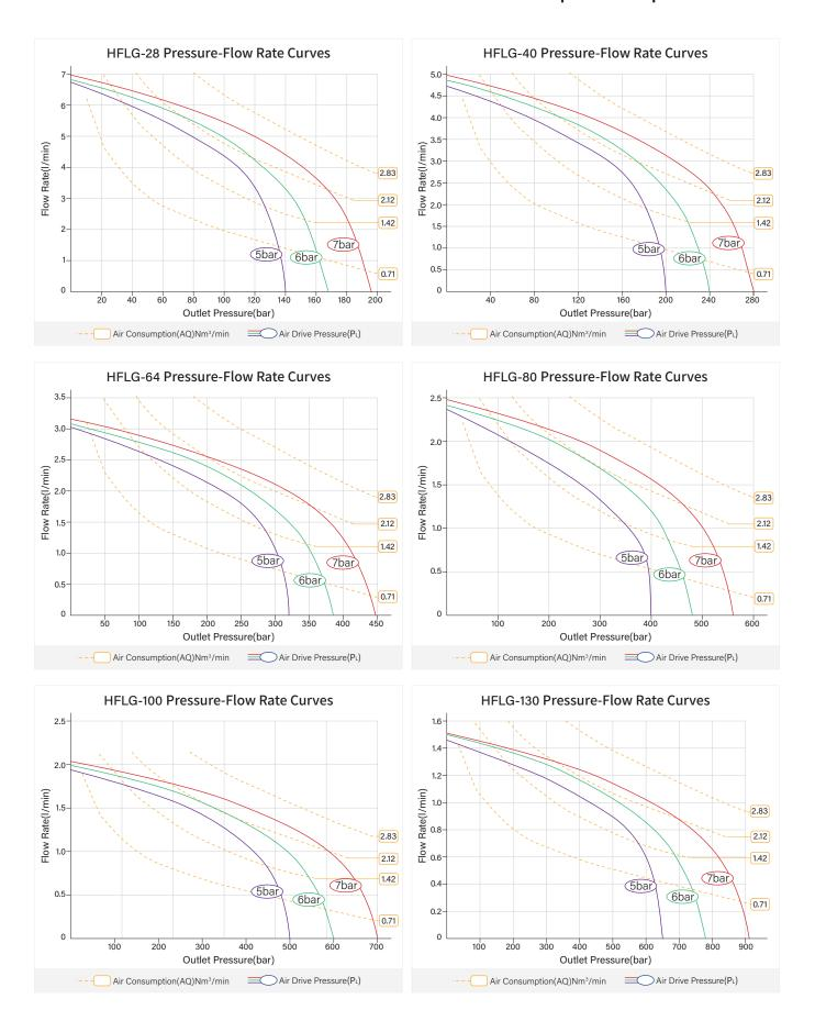
www.hifluid.com 16 Pressure-Flow Rate Curves
