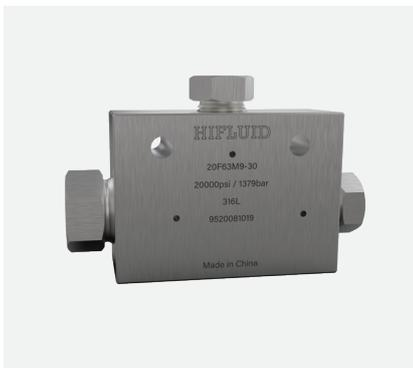
Angle Filters capture solid impurities to protect downstream equipment. Compared with Cup-Type Line Filters, the angle design allows element replacement without dismantling piping, making maintenance more convenient. Standard ratings: 5μm, 30μm, 56μm, which can be flexibly selected according to different operating requirements.
