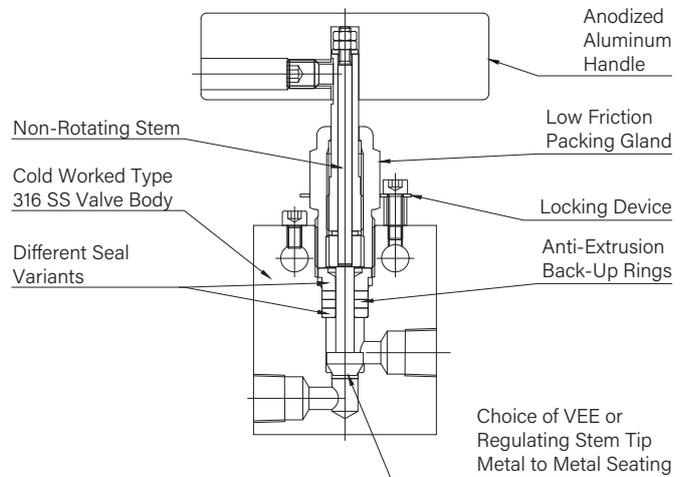
\* Cv values shown are for 2-way straight pattern vee stem valves. For 2-way angle patterns, increase the Cv value by 50%.
