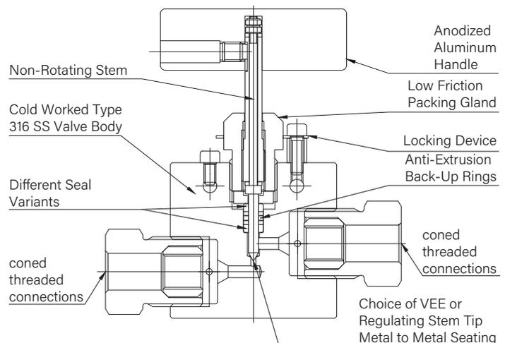
\* Cv values shown are for 2-way straight pattern vee stem valves. For 2-way angle patterns, increase the Cv value by 50%.
