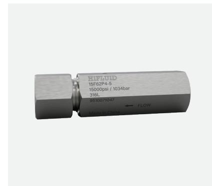
Cup-Type Line Filters capture solid impurities to protect downstream systems. The cup element provides a larger filtration area. Standard ratings: 5μm, 30μm, 56μm, which can be flexibly selected according to different operating requirements.
