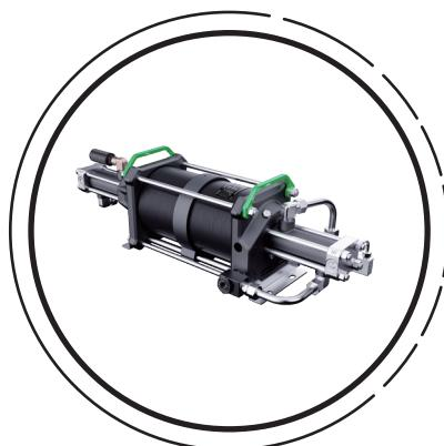
The HiFluid HFG Series air driven gas boosters use compressed air as the driving source to boost process gases to the required pressure. They are widely applied to oil-free compression of various industrial gases such as nitrogen, hydrogen, argon, helium, and methane, with working pressures up to 22,000psi.
