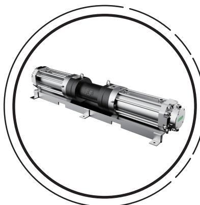
The HiFluid HFHG1 Series hydraulically driven gas boosters use low-pressure hydraulic oil as the driving source to boost process gases to the required pressure. The standard design supports a maximum working pressure of 17,000 psi, with special designs available for higher pressure requirements. These boosters are highly efficient for ultra-high-pressure and large-flow gas applications.
