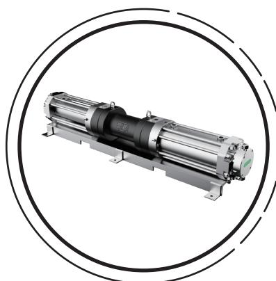
The HFHG1 series hydraulically driven gas boosters developed by HiFluid use low-pressure hydraulic oil as the driving source to pressurize process gases to the required pressure levels. The standard design supports a maximum working pressure of up to 120Mpa, with customized designs available for higher pressure requirements.
