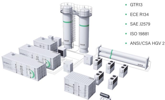
The Hydrogen Cylinder Hydrogen Cycle Test System, independently developed by HiFluid, is designed to evaluate fatigue life under extreme temperature conditions and varying hydrogen temperatures. The standard test pressure is 87.5MPa, with test environments ranging from -40°C to 85°C.
